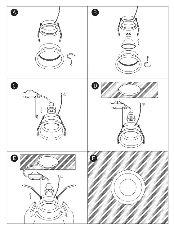
\*IP65 is the protection degree for the visible part of the fitting under the ceiling. The part of the fitting hidden in the ceiling is IP20.
